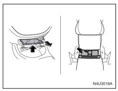
The front ashtray is located at the lower part of the center of the instrument panel. To remove the front ashtray for cleaning, open the ashtray fully, lift the inner case up and then pull it out.
